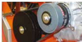
CENTRIFUGAL CLUTCH DEVICE (JUMBO P13 ONLY)
