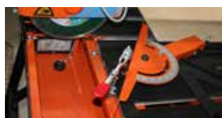
ANGULAR CUTTING GUIDE / RUBBER-COVERED TABLE
