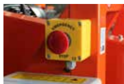
EMERGENCY PUSH BUTTON
