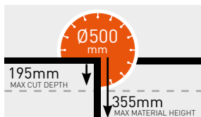
MAX CUT DEPTH - Ø500
