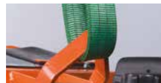
BUILT-IN LIFTING EYE
