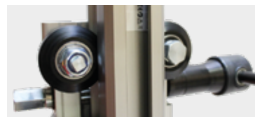
CARRIAGE GUIDING SYSTEM BY ROLLS.
