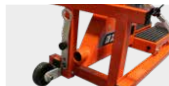
DUST EXTRACTION PORT Ø 40mm
