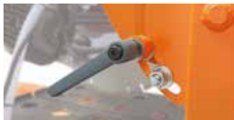
ADJUSTABLE CUTTING-DEPTH HANDLE
