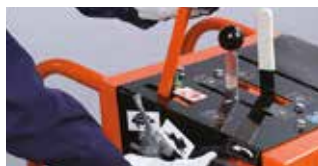
MANUAL OR HYDRAULIC RAISE & LOWER THE BLADE
