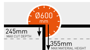
MAX CUT DEPTH - Ø600
